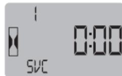
a) Press the button 3 times until display shows “SVC 1” icon and maintenance interval time.
