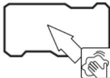
b) Remove protection from double-sided tape. Note: when removing the double-sided tape protector, make sure that the double-sided tape is not exposed to water or oil on both sides.
